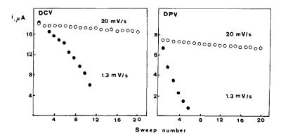
Figure 2 Study of the reproducibility of the voltammetric signal with the potential sweep rate;  $[D_3] = 1.3 \times 10^{-4} \text{ M}$ ,  $[\text{LiClO}_4] = 0.075 \text{ M}$  in methanol.
